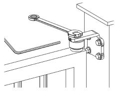
3) To adjust and fix the hinge, adjust the screw and dowel.
