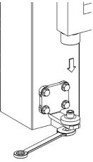
3) Adjust and fix the plate by means of the screw.
