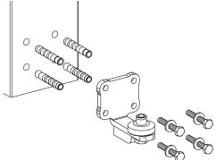
2) Position the hinge in its definitive position and mark the position of the holes; drill the post, insert the plugs, position and fix the hinge. Positioning the plate resting on the ground is recommended for greater security.
